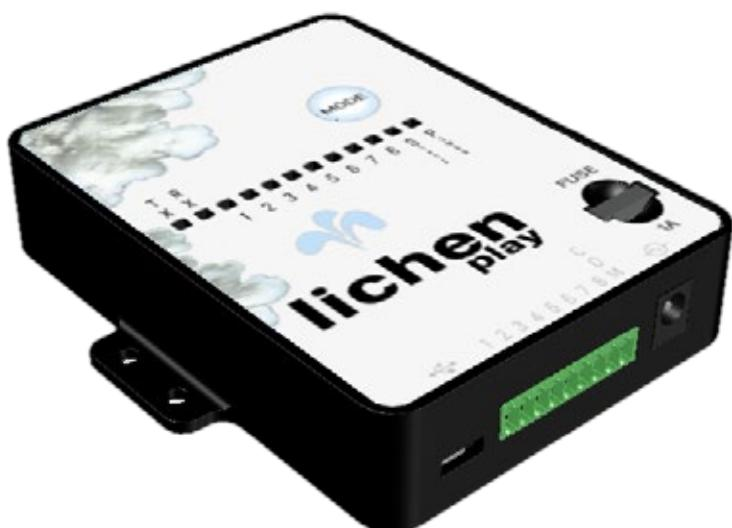
**Overlay:** Graphic overlays (often referred to as nameplates or faceplates) are printed material, with a decorative and practical design adhered to the surface of a product. Graphic overlays can be both cosmetic to visually enhance your product and brand, as well as functional to help make consumer interactions easy.
